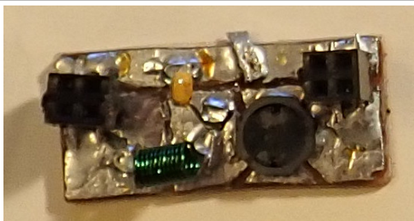
Figure 7: Old version of the board (2017). It has the female rectangular headers instead of SMA. Strange that I took this picture with the input at left.
